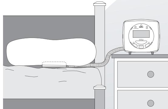
2. In the event of a fire, the pillow pad will vibrate and the unit will flash. The word 'fire' will also be present on the display.
