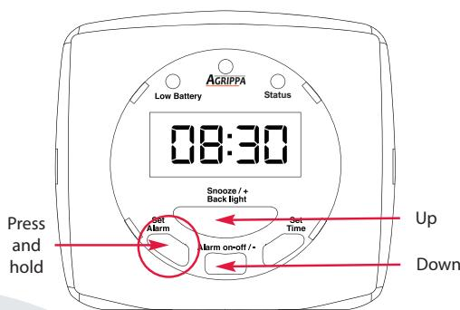
2. To enable/disable the alarm at any instant, press the 'Alarm on-off' button.
