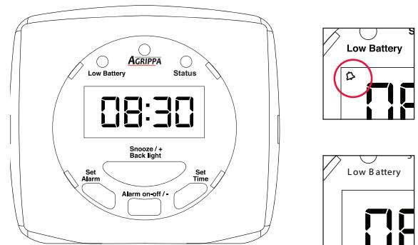
3. When the alarm triggers the pillow pad will vibrate. Pressing the 'Snooze' button will pause the alarm for five minutes.
