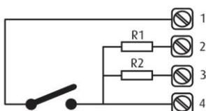
The ReSet Call Point will interface with most conventional fire alarm systems. It is fitted with two internal resistors 470 (R1) and 680 (R2) ohms. These are easily accessed through the installer terminals as illustrated.
